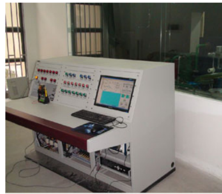
Fig. 6. Pump performance test-bed based on virtual instrument technique
